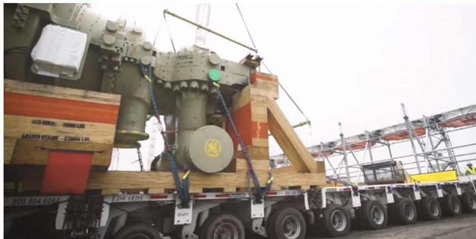
A GE turbine is hauled in for the Clear River Energy Center. | Invenery
